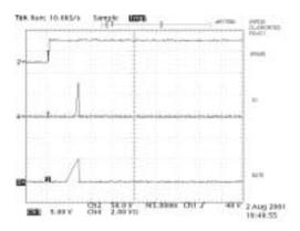
For most applications and pass elements, the HV100/HV101 provides adequate limiting of the maximum current to prevent damage without the need for any external components. The 2.5s delay of the auto-retry circuit provides time for the pass element to cool between attempts.
