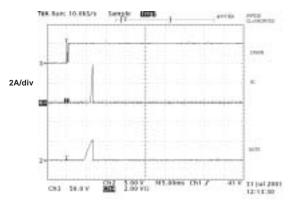
The maximum current that may occur during this period can be controlled by adding a resistor in series with the source of the MOSFET. The lower graph shows the same circuit with a 100m $\Omega$  resistor inserted between source and V<sub>NN</sub>. In this case the maximum current is 25% smaller.
